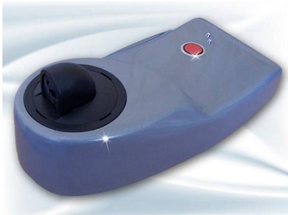
Figure 3. The Gas Discharge Visualization (GDV) device. Under the optic plate (glass), a high intensity and high frequency electric field stimulates a fingertip corona discharge, which is photographed by a CCD camera. A guide is placed on the glass, to help position the fingertip correctly and screen out environmental light sources. During the measurement, it is recommended to wear a cloth around the hand, similar to a small cloak, as a further screen from external light. Picture retrieved from gdvusa.org
